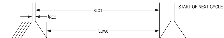
1-Wire WRITE-ZERO TIME SLOT
