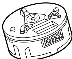
Right angle version (shown here with press fit/adhesive mount hub option)
