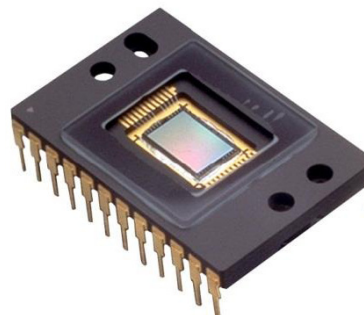
Figure 1. KAF-0402 Full Frame CCD Image Sensor
