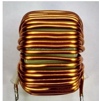
The chosen core material is HIGH FLUX from Chang Sung Corporations (CSC), which has an excellent DC bias and good core loss behavior. The part number is CH270060E18. The outer diameter of the core is 27 mm with a height is 19 mm.
