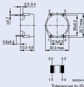
Tolerances to ISO 2768-C unless otherwise noted. Dimensions in mm.
