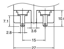
Remark: Power switching contact type has .250 Quick-connect terminal and signal switching contact type has .110 Quick-connect terminal.
