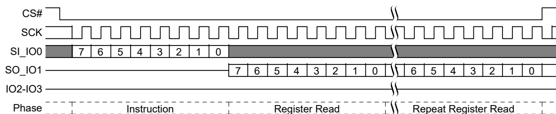
Figure 56. Read Configuration Register (RDCR) Command Sequence
