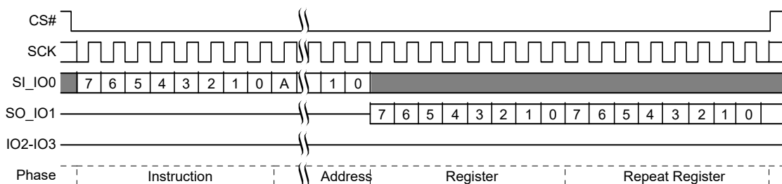
Figure 110. PPB Read Command Sequence
