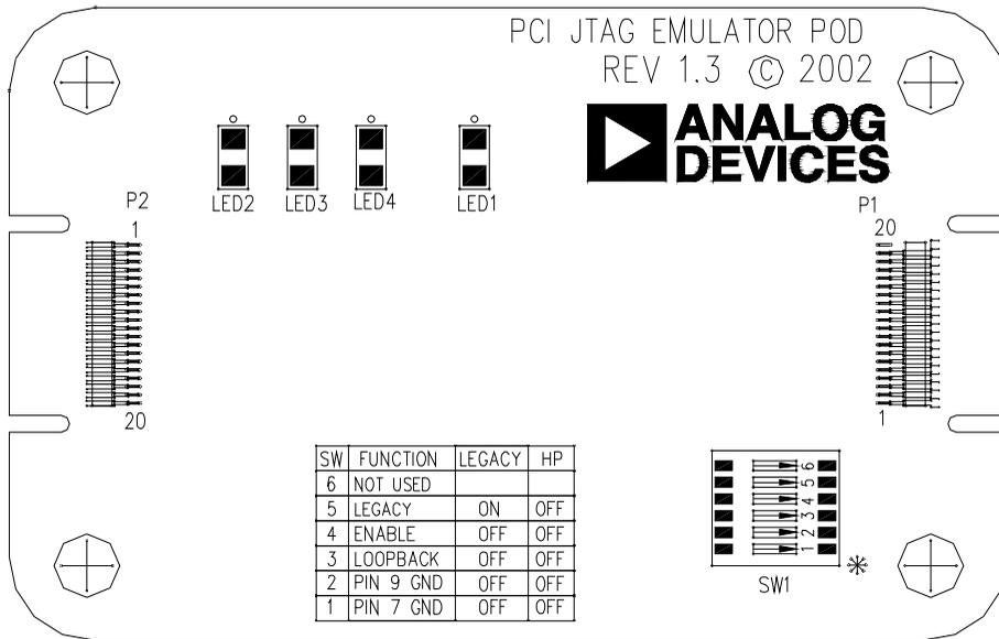
Figure 1-7. Auto Detection Switch Setting for HPPCI-ICE Pod
