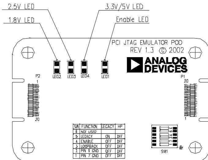
Figure 2-1. Pod LEDs
