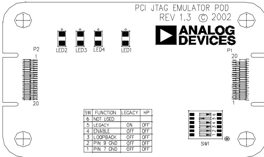
Figure 1-6. Legacy Switch Setting for HPPCI-ICE Pod
