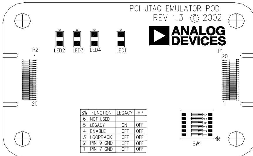
Figure 1-5. Default Switch Setting for HPPCI-ICE Pod
