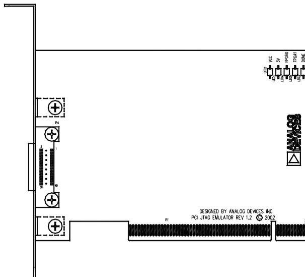
Figure 2-2. Board LEDs
