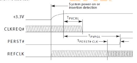
Note:  $T_{PVCRL}$  is measured from the later rising edge of +3.3V.
