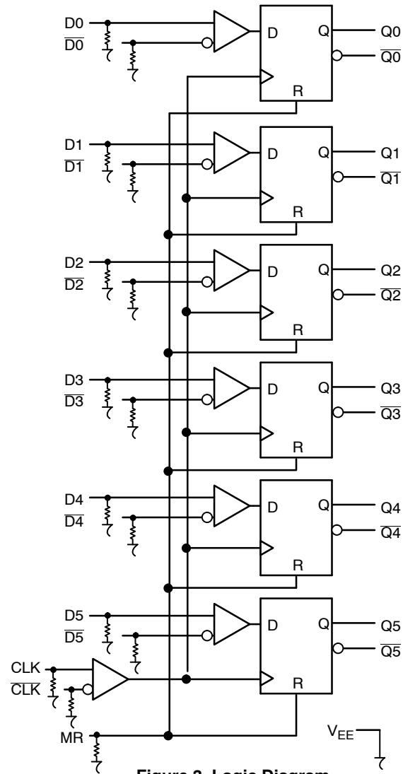
**Figure 3. Logic Diagram**
