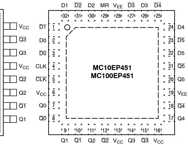
**Figure 2. QFN-32 Pinout (Top View)**
