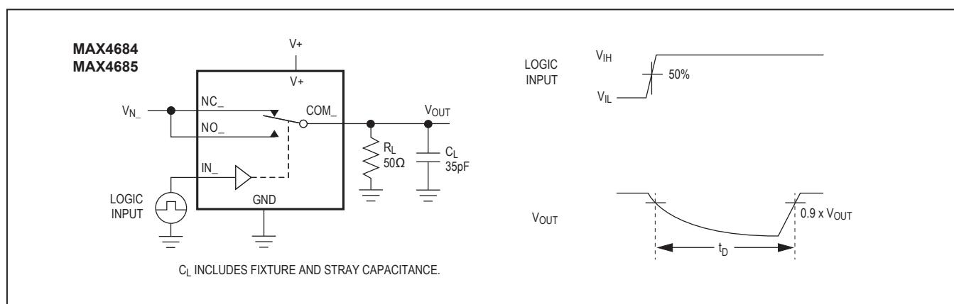
Figure 3. Break-Before-Make Interval
