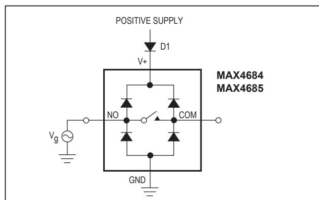
Figure 1. Overvoltage Protection Using Two External Blocking Diodes
