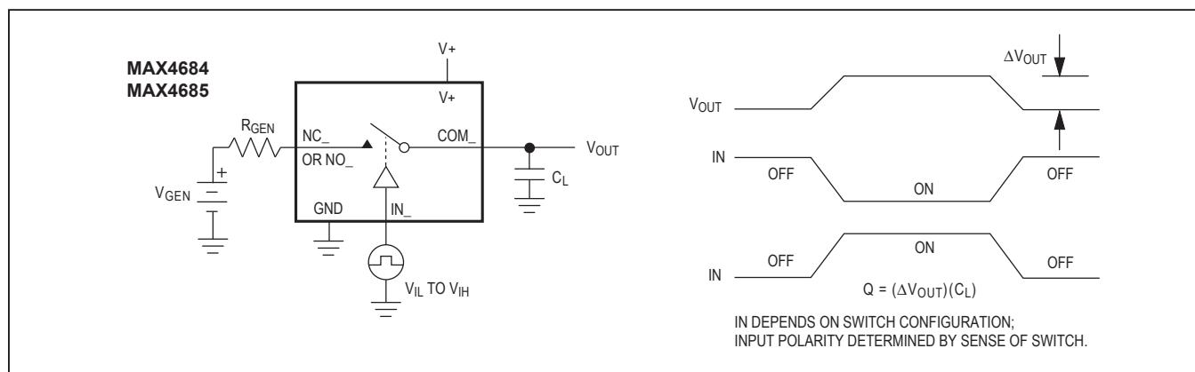
Figure 4. Charge Injection
