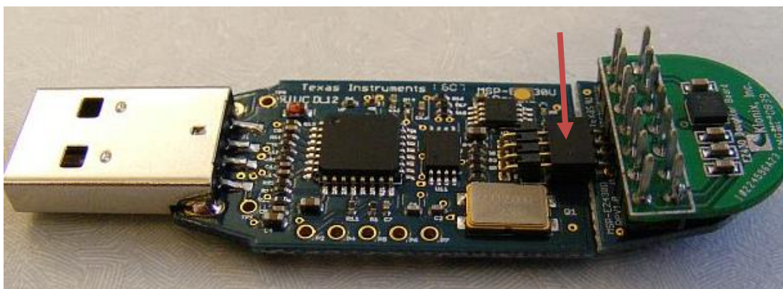
Figure 2: eZ430-F2013 development kit with 4-pin target board connector
