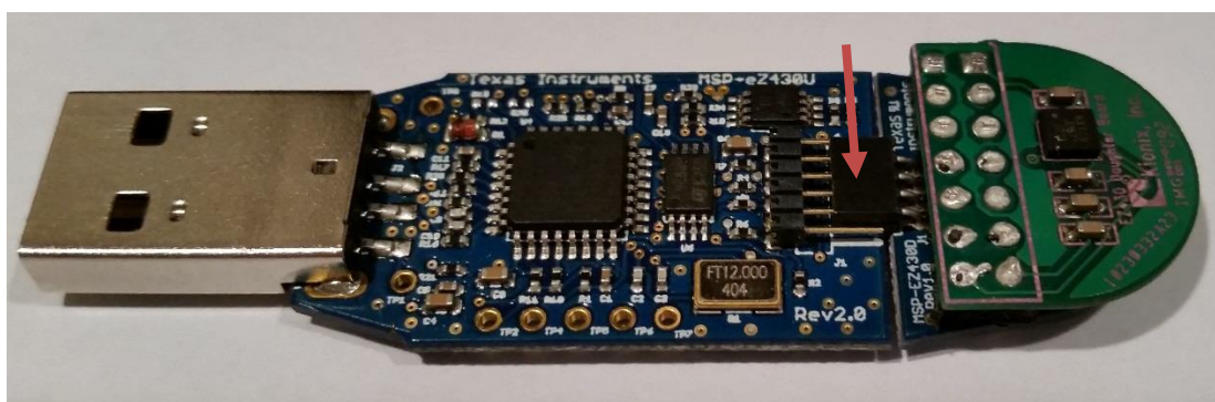
Figure 3: eZ430-F2013 development kit with 6-pin target board connector
