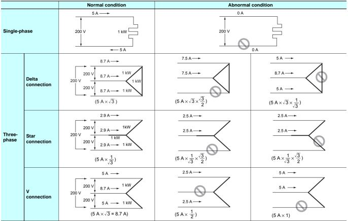
Note: This is the current for when a 200-V, 1-kW heater is used for single-phase or three-phase operation.
