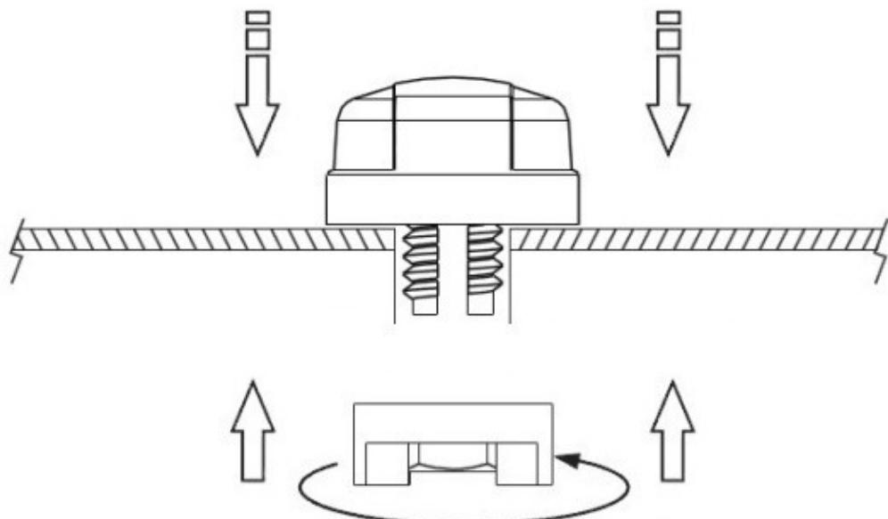
Recommended torque for Mounting is  $24.5\text{N}\cdot\text{m}$
