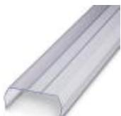
Cover profile, for covering terminal strips, snapped onto APT-ME cover profile carrier or APH-ME end bracket. A cover profile carrier should be positioned at the ends and at intervals of around 40 cm. Length supplied: 1 m
