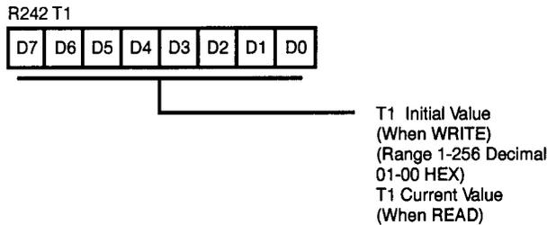
Figure 23. Counter Timer 1 Register (F2H: Read/Write)
