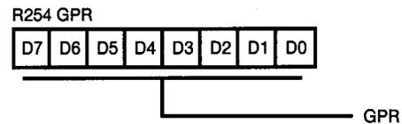
**Figure 35. General-Purpose Register (FEH: Read/Write)**
