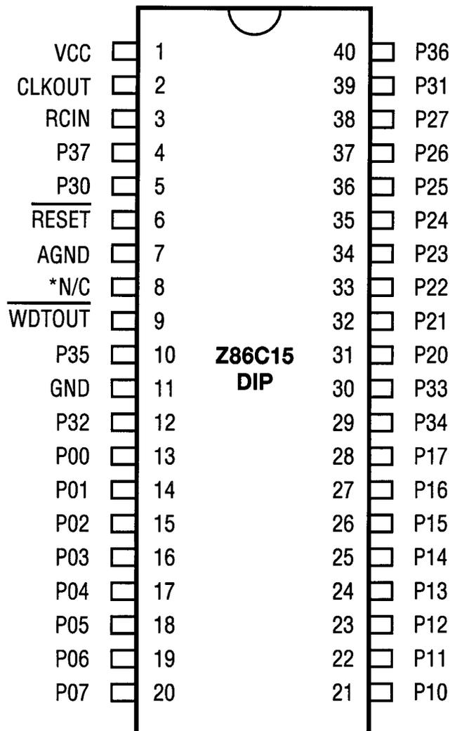
**Note:** Pin 8 is connected to the chip, although it is used only for testing. This pin **must** float.
