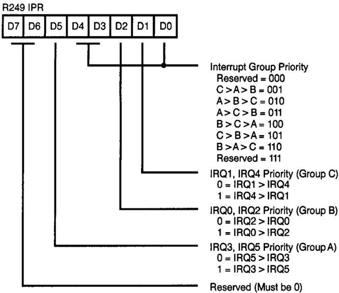
**Figure 30. Interrupt Priority Register (F9H: Write Only)**
