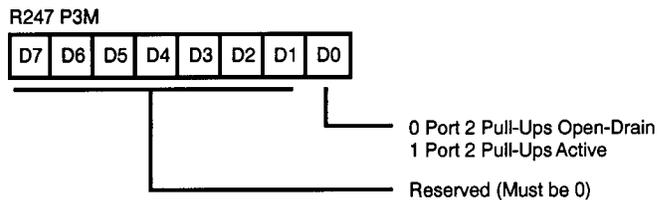
Figure 28. Port 3 Mode Register (F7H: Write Only)
