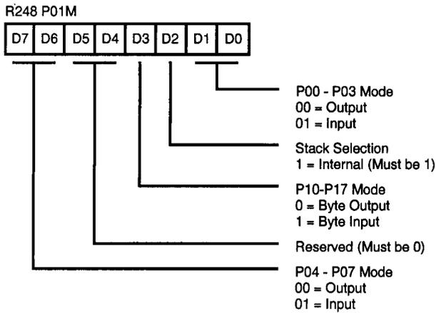
**Figure 29. Port 0 and 1 Mode Register (F8H: Write Only)**
