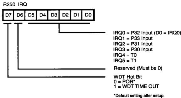
**Figure 31. Interrupt Request Register (FAH: Read/Write)**
