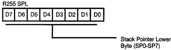
**Figure 36. Stack Pointer
