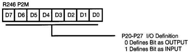
Figure 27. Port 2 Mode Register (F6H: Write Only)
