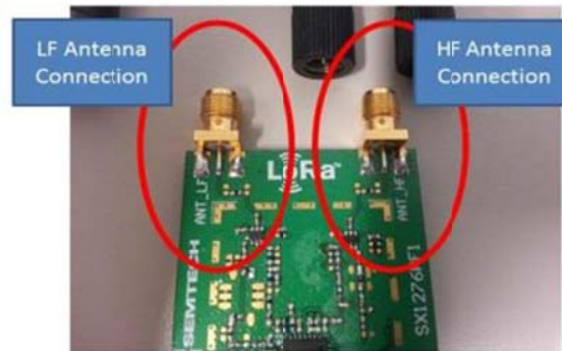
Figure 6: LF and HF Antenna Connection
