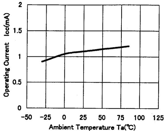
**Battery Saving Operating Current vs. Temperature**
