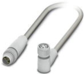
Sensor/Actuator cable, 3-position, PP-EPDM halogen-free, gray RAL 7035, Plug straight M8, on Socket angled M8, with 2 LEDs, Cable length: 0.6 m, Hygienic design, with plastic knurl
