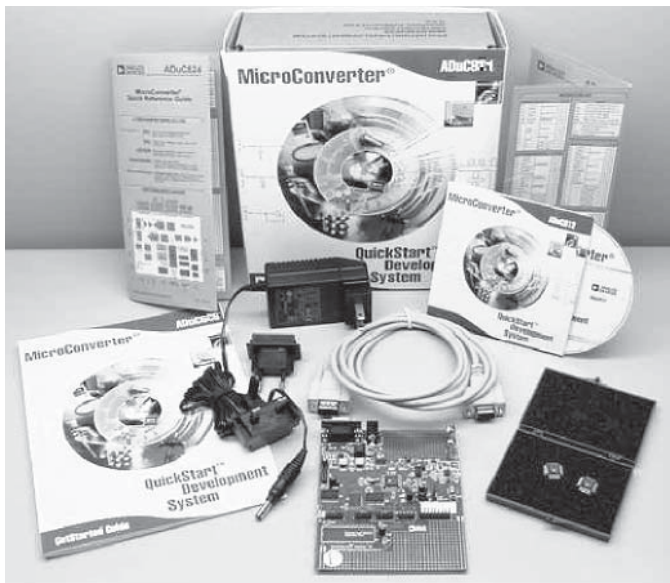
Figure 53. Components of the QuickStart Development System
