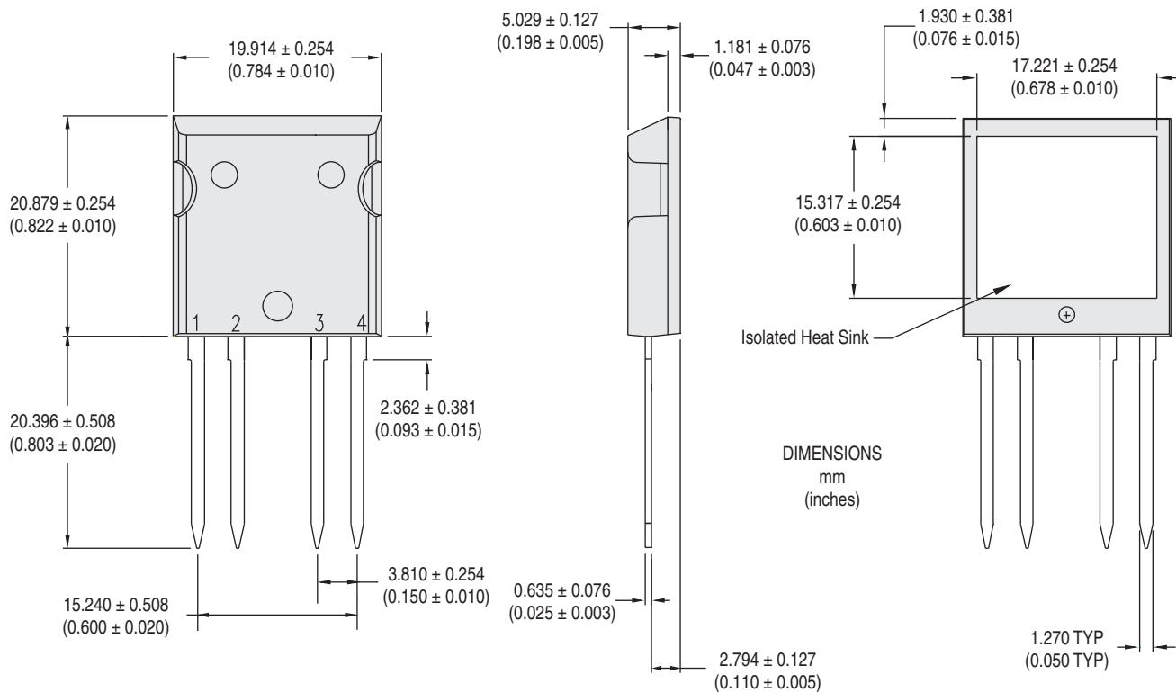
NOTE: Back-side heat sink meets  $2500V_{rms}$  isolation to the pins.
