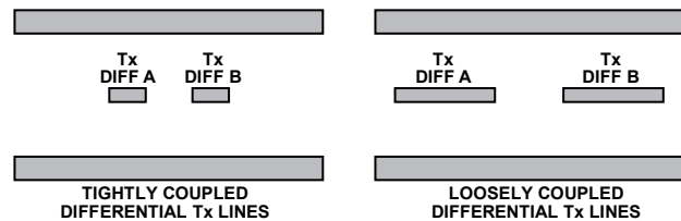
Figure 78. Tightly Coupled vs. Loosely Coupled Differential Traces
