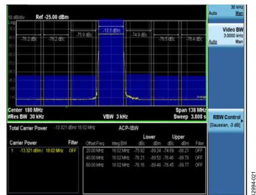
Figure 20. 1C 5 MHz Bandwidth LTE ACLR Performance, IF = 180\text{ MHz} , f_{DAC} = 1966.08\text{ MHz}
