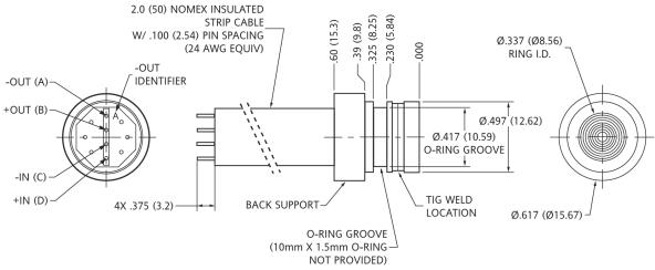
**Note:** Non-concentricity effects at the diaphragm weld area may cause runout of up to  $\pm 0.006$  in between the upper and lower portions of the sensor body. (It is recommended to use a counter bore to mate with this device to allow for this non-concentricity).
