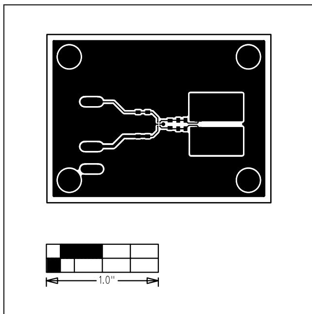
Figure 3. MAX9928 EV Kit PCB Layout—Component Side
