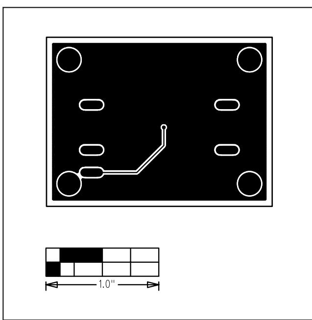
Figure 4. MAX9928 EV Kit PCB Layout—Solder Side
