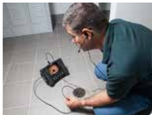
Record video with audio during pipe inspections
