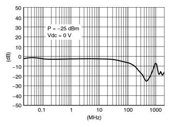
Figure 2. Insertion Loss Characteristics
