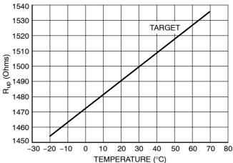
Figure 4. R<sub>up</sub> versus Temperature
