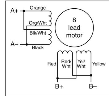
Eight lead motor connected in SERIES to a bipolar drive.
