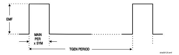
A single cycle of the main generator (i.e. a single pulse) will now be output at the default frequency of 1 kHz, so a 1000:1 duty cycle has now been achieved. Move the cursor to the TGEN period field with the **FIELD** keys and increase the period using the rotary control; although it will be difficult to see on the oscilloscope, the 1  $\mu$ s pulse width is maintained down to milliHertz repetition rates, i.e. an extremely small duty-cycle.
