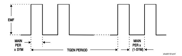
Set TGEN to 1.00 ms again (1 kHz) and the burst count to 2; this will give the waveform shown. The pulse width and interval between successive pulses is determined by the main generator frequency and symmetry; the pulse width will be PER multiplied by SYM, and the pulse low time will be PER multiplied by (1-SYM). The repetition rate of the bursts remains determined by the TGEN period.
