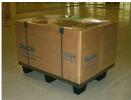
Fig. 1: Proper packing of relays for transportation
