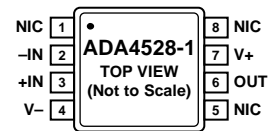
Figure 1. ADA4528-1 Pin Configuration, 8-Lead MSOP
