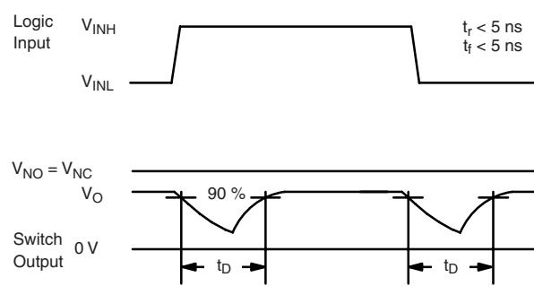
**Figure 2. Break-Before-Make Interval**
