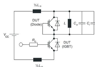
Figure E. Dynamic test circuit
