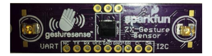
Note the labeled connections are shown here—it is important that the FTDI cable goes is connected to the UART portion of the pin-out. I2C connections are for only the 3 pins on the right, as well as using VCC and GND connections to power the sensor.
