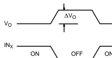
**FIGURE 4.** Charge Injection
