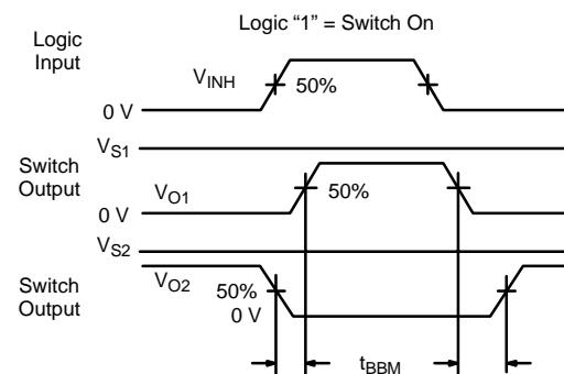
**FIGURE 3.** Break-Before-Make SPDT (DG387B, DG390B)
