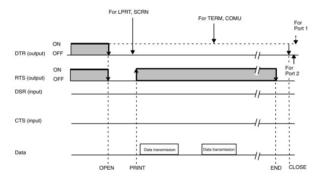
Note 1. If the DSR or CTS signal is disabled, these signals will be ignored. However, if the CTS signal to port 2 needs to be disabled, either pull it HIGH or connect it to the RTS signal. If the RTS signal is selected as the valid signal by the OPEN command, the RTS signal will remain HIGH. The RTS signal goes low when the CLOSE command is executed.
