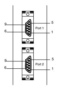
Plug: XM2A-0901 (OMRON) or equivalent. Applicable Connector Hood: XM2S-0901 (OMRON) or equivalent. (Two plugs and two hoods are supplied with the ASCII Unit.) Cable Length: 15 m
