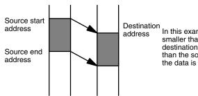
In this example, the source start address is smaller than the destination address and the destination address is equal to or smaller than the source end address. Consequently, the data is not transferred correctly.
