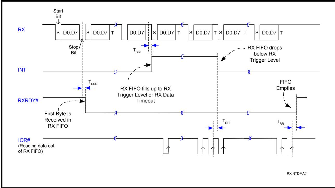
FIGURE 21. RECEIVE READY & INTERRUPT TIMING [FIFO MODE, DMA ENABLED] FOR CHANNELS A & B
