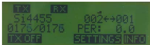
Figure 15. Running PER Test (TRx Mode)
