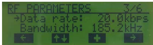
Figure 9. Menu Page: RF Parameters 3/6 (Modulation is OOK)
