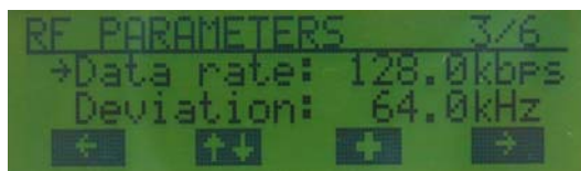
Figure 8. Menu Page: RF Parameters 3/6 (Modulation is 2GFSK)
