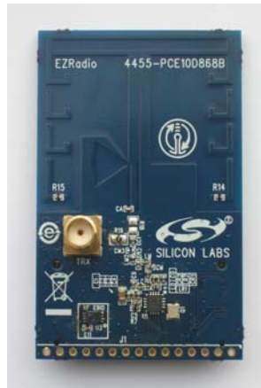
Figure 2. Si4455 RF Pico Board—868 MHz (P/N 4455-PCE10D868B)
