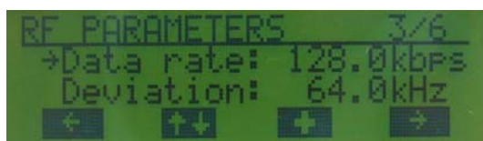
Figure 8. Menu Page: RF Parameters 3/6 (Modulation is 2GFSK)
