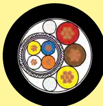
Structure Hybrid cable
