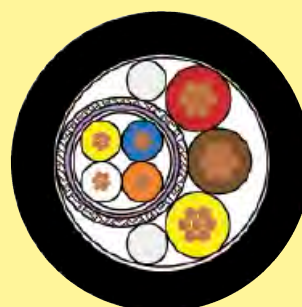
Structure Hybrid cable
