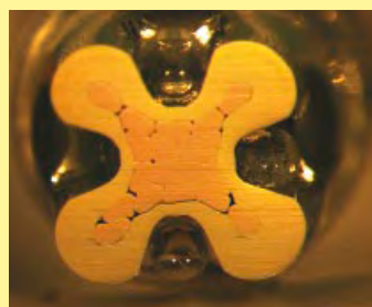
Crimp-cross section HARTING crimp profile
