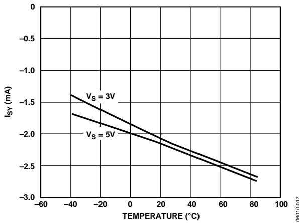
Figure 20. I<sub>SY-</sub> vs. Temperature
