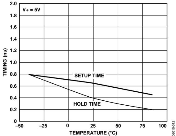
Figure 15. Latch Setup and Hold Time vs. Temperature
