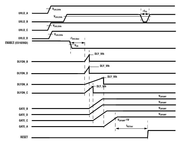
FIGURE 6. ES1020QI TURN-ON AND GLITCH RESPONSE TIMING DIAGRAM
