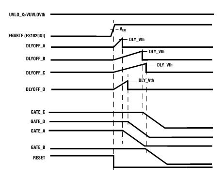
FIGURE 7. ES1020QI TURN-OFF TIMING DIAGRAM
