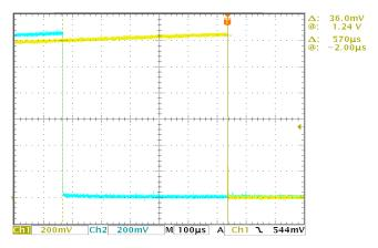
FIGURE 10. CAPACITOR TIMING MISMATCH
