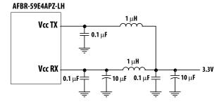
**NOTE** Inductors should have less than  $1-\Omega$  series resistor per MSA.
