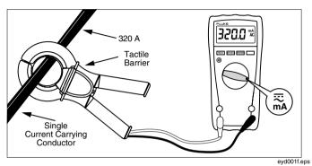
Figure 1. Current Measurement
