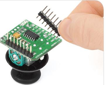
Turn the board upside down so that the bottom side is facing you upwards. Place shorter pins of the header into the appropriate soldering pads.
