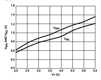
FIGURE 15. DIGITAL SWITCHING POINT vs SUPPLY VOLTAGE
