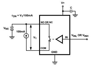
FIGURE 5. ron TEST CIRCUIT
