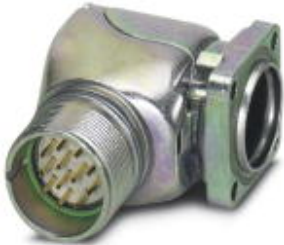
Device connector, front mounting, angled rotatable, Screw locking, M23, number of positions: 6, type of contact: Pin, Solder connection, Axial O-ring, 4x Ø 3.2, shielded: yes
