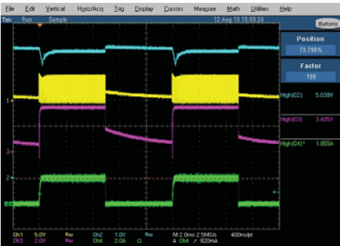
Figure 26. 100 Hz PWM dimming function
