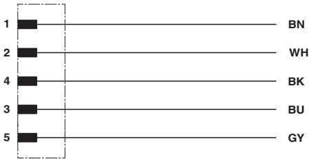
Contact assignment of the M12 plug and the M12 socket
