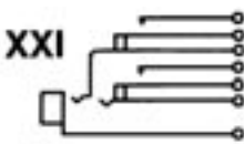
Double open circuit. Isolated switching—separate "make" circuits on both tip and ring. (J2-2A).
