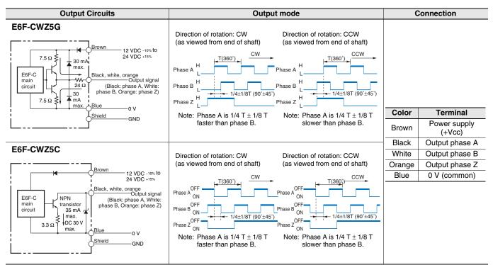
Note: 1. The shielded cable outer core (shield) is not connected to the inner area or to the case.
